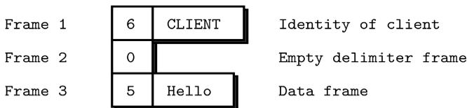
Figure 36. Message Delivered to Worker
